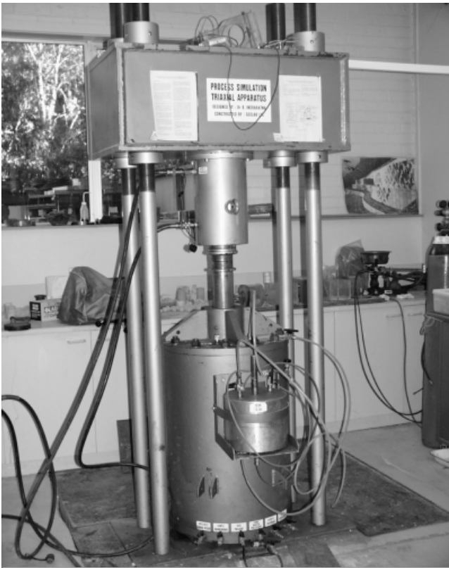
Fig. 2. Large-scale triaxial apparatus built at University of Wollongong, Australia
