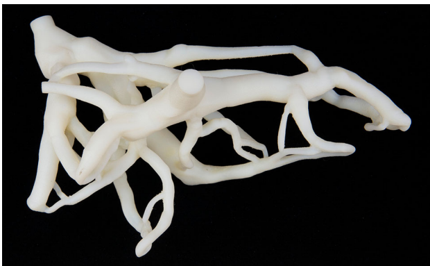
Fig. 12 3D printed liver vascular system using ABS
