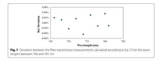
a slightly higher stray light. This additional stray light leads to a higher signal. In case of the combined measurement with two filters simultaneously positioned in the beam path, this stray light occurs just once. In case of the two individual measurements, this stray light is measured twice, thus a deviation of 0.3% between the measurements occurred. For the integrating sphere, the back reflection is almost completely diminished.
