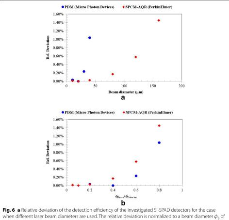
approx. 20  $\mu$ m; **b** relative deviation of the detection efficiency as a function of the diameter ratio of the beam and the active area of the investigated Si-SPAD detectors
