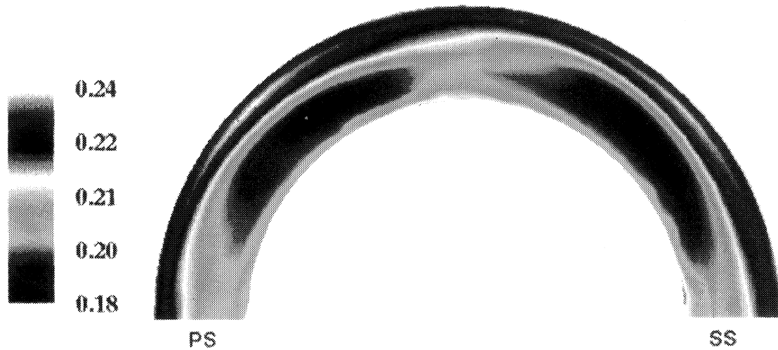
FIGURE 5 Consortium baseline impeller inlet laser survey (nondimensional tangential velocity C_u ).
