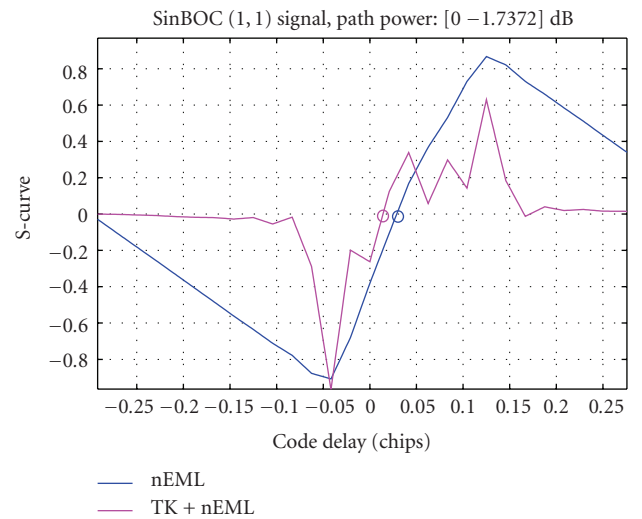
FIGURE 4: S-curve in SinBOC(1,1)- modulated 2 path Rayleigh channel model, path delay: [0 0.0833] chips, path power: [0-1.7372] dB, C/N_0 : 100 dB-Hz, BW: 24 MHz.
