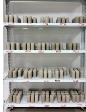
FIGURE 3: Samples curing in air.
