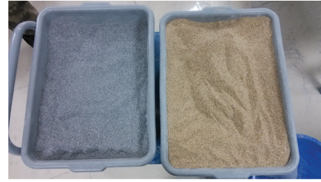
FIGURE 1: Raw material: barite sand and quartz sand.
