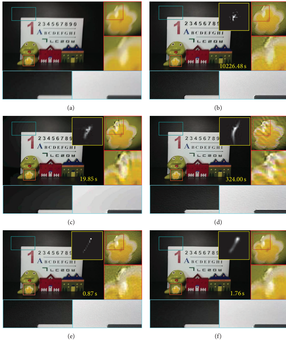
FIGURE 5: Comparison of different image restoration methods: (a) input motion-blurred image, (b) Fergus’s method [3], (c) Cho’s method [7], (d) Shan’s method [5], (e) Šindelář’s method [16], and (f) the proposed method.
