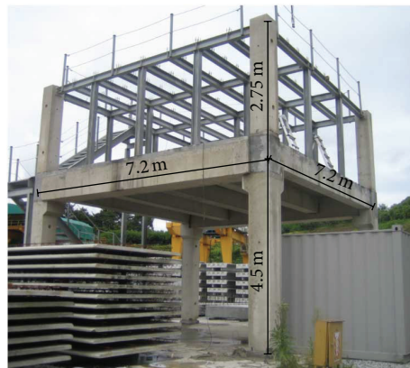
FIGURE 2: 1/2 scale model manufactured by using mass-based scaling method.
