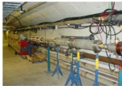
FIGURE 9. Inductive inserts in the Fermilab Booster.
