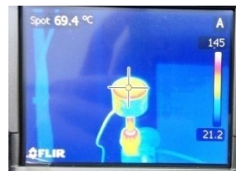
Fig. 6. Real – time monitoring of PLA disk with T400 thermal imaging camera.
