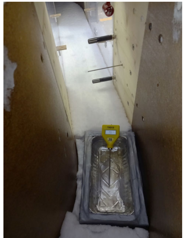
Fig. 6. The water bowl was placed in the snow at the start of the main test section. The bowl was insulated with styrofoam.
