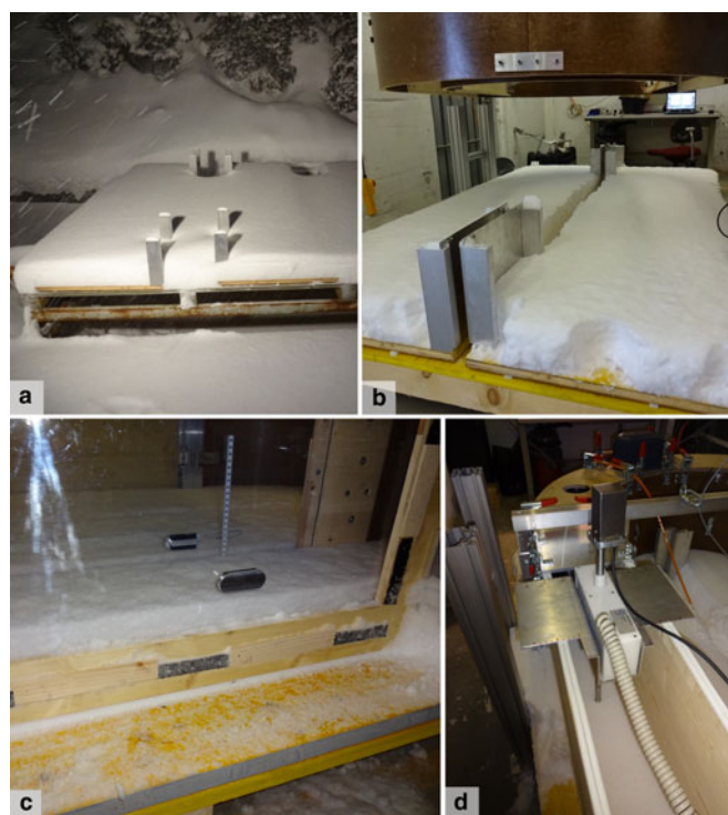
Fig. 2. Operation of the wind tunnel. (a) Snow is collected on trays and (b) arranged below the wind tunnel. (c) Then, the wind tunnel is lowered into the snow. (d) The SnowMicroPen (SMP) during a measurement. The SMP is the main instrument.
