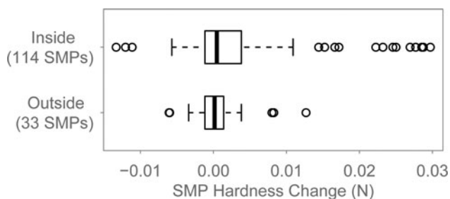
Fig. 8. Comparison of the SMP hardness change in wind periods without drifting and the SMP hardness change measured outside the wind tunnel during the same time periods.
