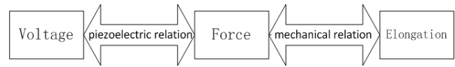
Figure 4. Internal relations of the piezoelectric actuator (no sequence between these two relations).
