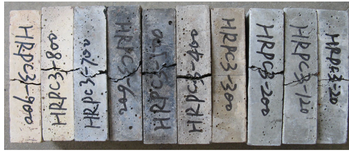
Fig. 4 Flexural failure modes of HRPC after elevated temperatures.
