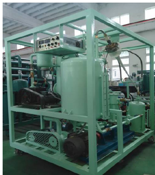
Fig. 2 Test device of three-field for emulsified oil's dehydration
