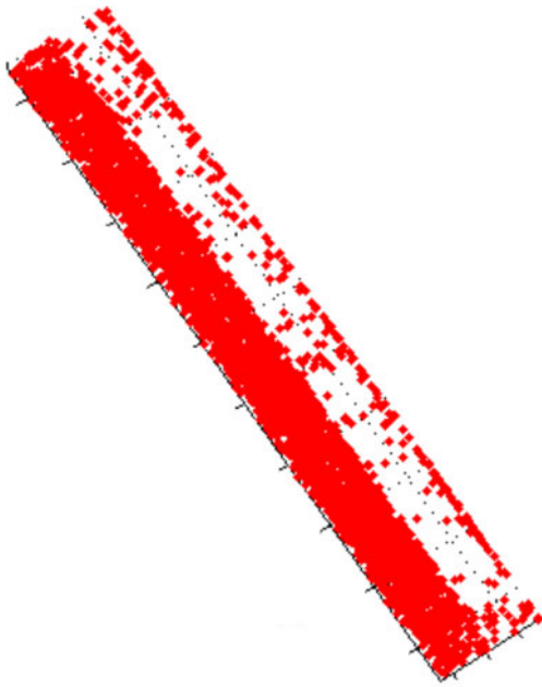
Fig. 1 Example of an aspect class for a simple two slope roof; spread and edge points are clearly visible
