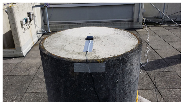
Fig. 2 u-blox M8T patch antenna placed on concrete pillar at the TU Delft GNSS observatory on top of the NMI building in Delft
