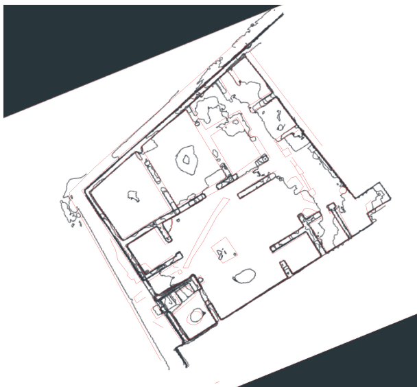
Figure 7. Overlap of the plants produced with total station (red) and with the 3D model (black)
