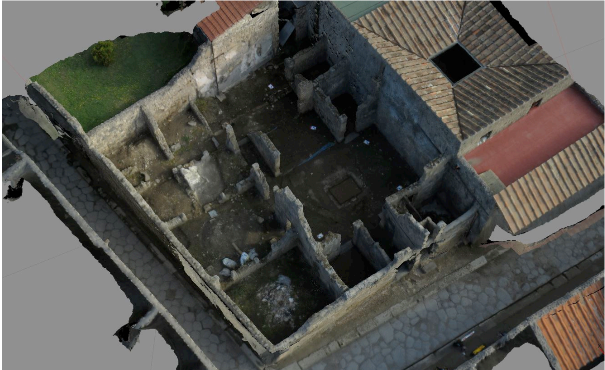
Figure 5. 3D model of Domus of Stallius Eros obtained by drone photogrammetry (top view)
