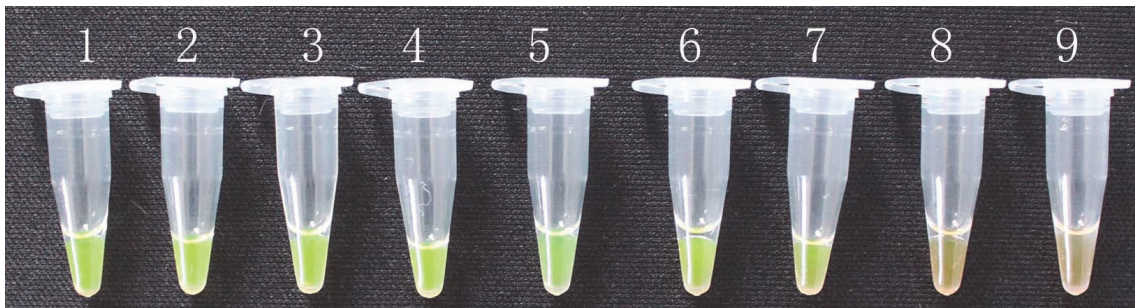
FIGURE 5: Limit of detection of LAMP assay. Tubes 1–9: nine 10-fold dilutions of purified DNA with concentrations ranging from 1 fg to 100 ng per microliter (tubes 1 to 9 in order) were tested. The limit of detection of LAMP assay was 0.1 \text{ pg} \cdot \mu\text{L}^{-1} .
