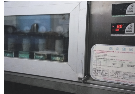
FIGURE 2: Experimental dies with specimen in the temperature box.
