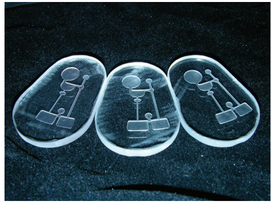
FIGURE 4: Centrifugal microfluidic chips with different widths of main channel.
