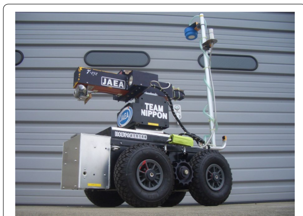
Fig. 6 JAEA-3 robot equipped with gamma imaging and measurement device
