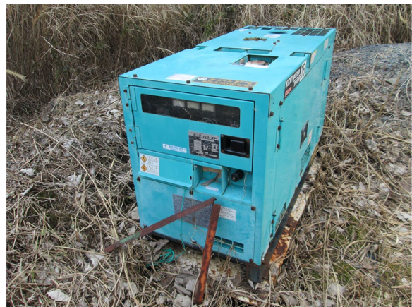
Fig. 5 Diesel drive electric generator
