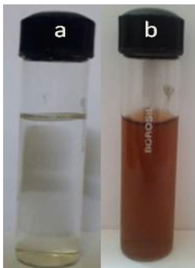
Fig. 1 Biosynthesis of AgNPs using D. montana : a stem bark extract of D. montana and b AgNPs
