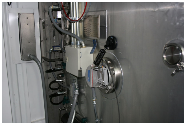
Fig. 9. Transmitter unit of a wireless system mounted at a site glass on a production-scale IMA Life freeze dryer by means of a suction cup
