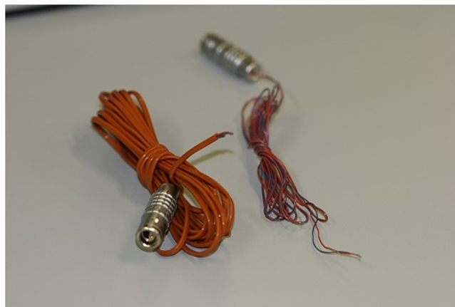
Fig. 3. The thermocouples shown here are representative of thermocouples commonly used in a production environment for product temperature measurement
