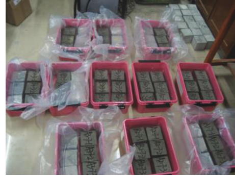
FIGURE 1: Concrete specimens exposed to drying-wetting cycles with sulfate attack.
