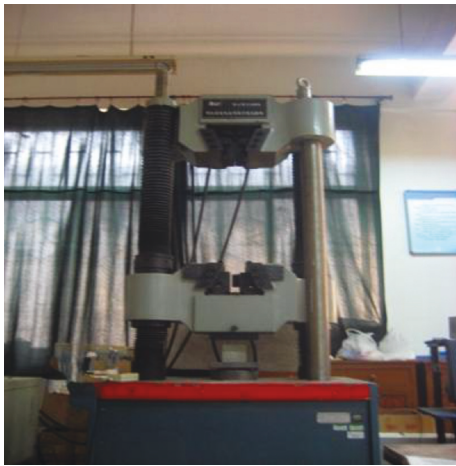
FIGURE 4: WAW3100 electrohydraulic servo testing system.
