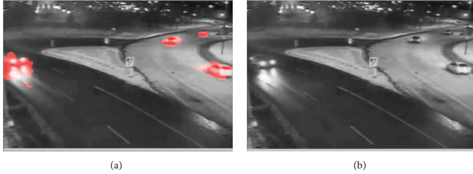
FIGURE 19: Segmentation of moving cars in the “winter street video” based on detected motion. (a) Motion detected by the phase-based motion detection algorithm. (b) Motion detected using optic flow algorithm [4] (see Supplementary Videos S11a and S11b for full videos).
