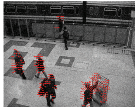
FIGURE 15: Phase-based motion detection applied on the “train station video” with added Gaussian white noise (see Supplementary Video S7 for full video).
