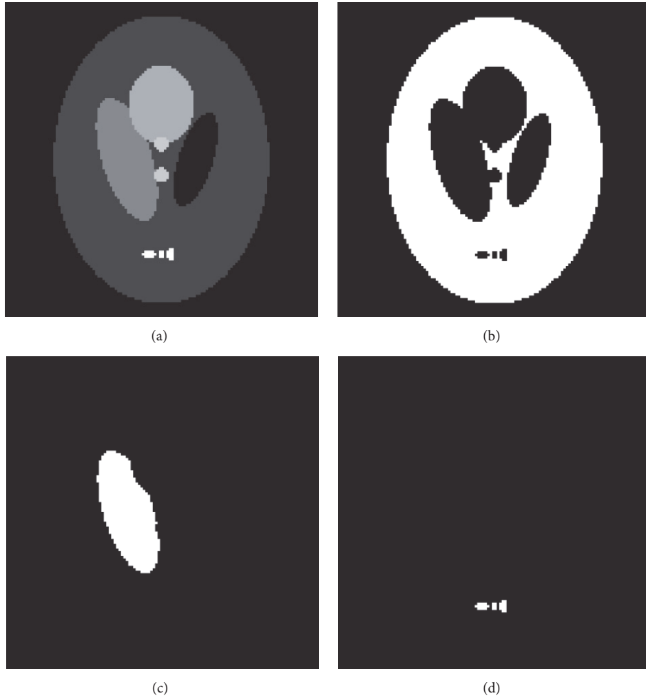
FIGURE 1: Shepp-Logan phantom with 128 \times 128 grids: (a) Shepp-Logan phantom, (b) background, (c) low-activity ROI, and (d) high-activity ROI.
