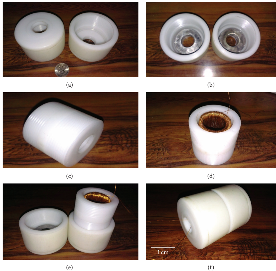
FIGURE 11: Fabrication of prototype-2: (a) Teflon capacitive energy harvester's holder caps, (b) capacitive energy harvesters placed in screwed holder caps, (c) screwed Teflon housing for inductive energy harvester, (d) inductive energy harvester placed in the main housing, (e) capacitive energy harvester holder cap screwed on the main housing, and (f) assembled prototype-2.
