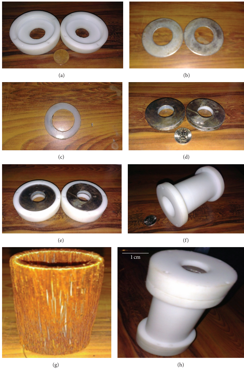
FIGURE 10: Fabrication of prototype-1: (a) capacitive energy harvester holder caps, (b) annular mild steel conductive plates, (c) Teflon spacer, (d) assembled capacitive energy harvesters, (e) capacitive energy harvesters in Teflon holder caps, (f) Teflon housing for inductive energy harvester, (g) copper wire wound around the cylindrical steel core, and (h) assembled prototype-1.
