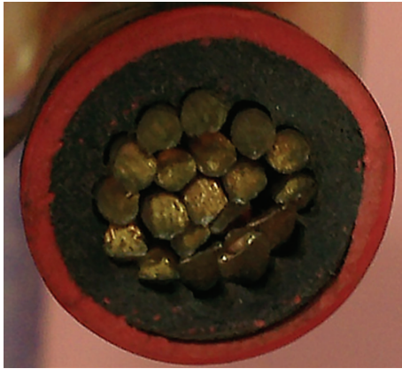
FIGURE 2: Single-core insulated cable for electrical power transmission.
