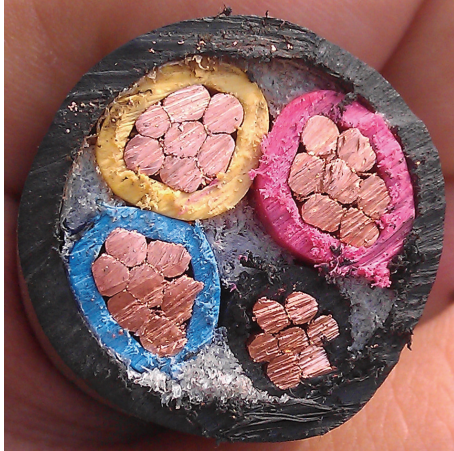
FIGURE 6: Three-core insulated cable for electrical power transmission.
