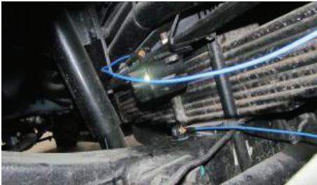
FIGURE 3: Accelerometer location of the chassis.
