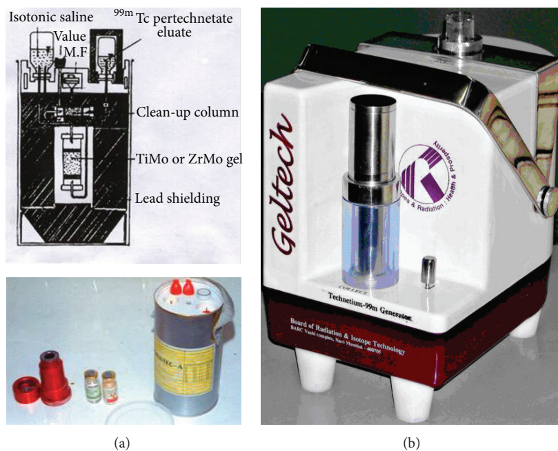
FIGURE 10: Typical chromatographic gel-type ^{99m}\text{Tc} generators (dual column systems compose of a ZrMo ( ^{99}\text{Mo} ) gel column coupled with a purification acidic-alumina column): (a) Gelutec-A ^{99m}\text{Tc} -generator manufactured by NRI (Vietnam); (b) Geltech ^{99m}\text{Tc} -generator by BRIT (India). (Note: no ^{99m}\text{Tc} -concentration is available in these generator systems. In Gelutec-A system, two alumina columns are installed in parallel and a selector/valve is inserted between them to direct the ^{99m}\text{Tc} eluate from the gel column being passed over each column for 5 consecutive purification/elutions) [2, 57, 59, 60, 103].
