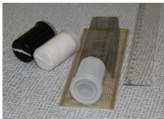
FIGURE 4: Cylindrical cotton wool filled plastic containers saturated with probe liquids attached to a horizontal glass slide covered with a powdered material used in “the thin layer wicking technique” to determine CA of the model materials (adapted after [7]).
