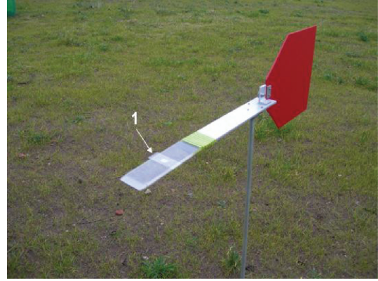
FIGURE 2: Natural dust deposition sampler system with a horizontal deposition plate to collect particles (1), self-oriented to the wind direction by wing (adapted after [6]).
