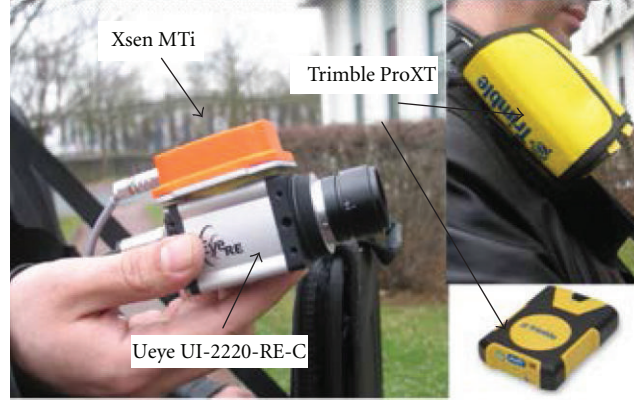
FIGURE 1: Sensor components of our Hybrid tracker.
