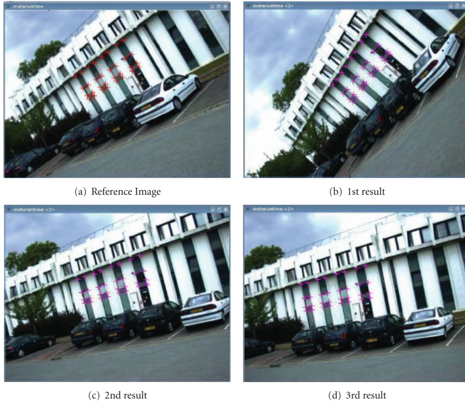
FIGURE 9: Matching results for automated initialization approach, case of the coplanar points.
