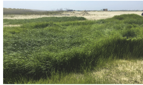
FIGURE 17: View of the section treated with coffee sludge on the 180th day of the field test.
