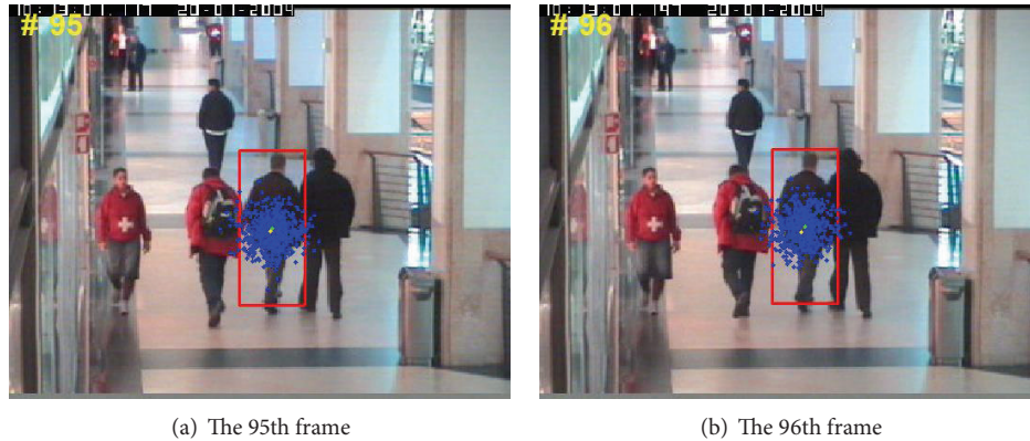
FIGURE 5: Tracking results in ThreePostShop2cor with Weight-Selection strategy (green: result of SR, yellow: result of PF, blue: the sampled particles, and red: the final tracking result).
