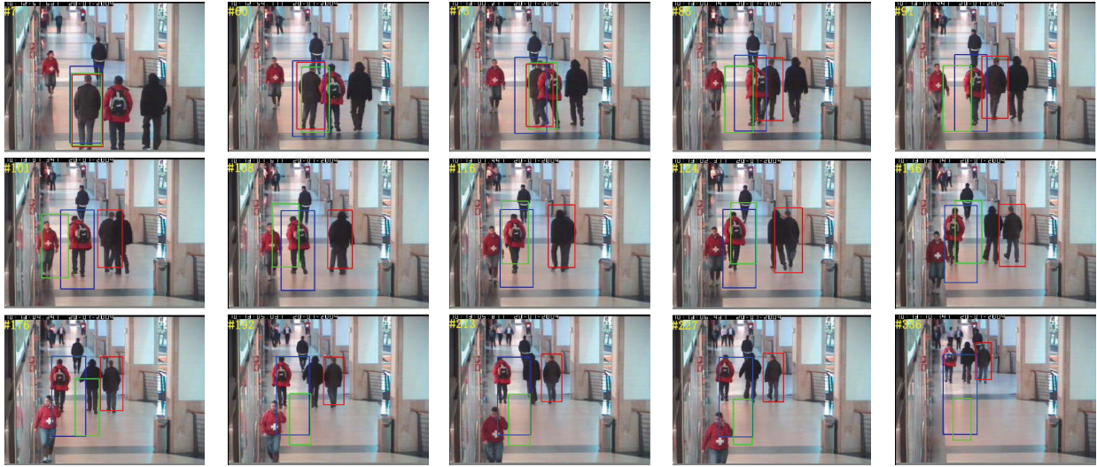
FIGURE 7: ThreePastShop2cor: the challenges are occlusions and pose variation (red: the proposed method; blue: TLD method; and green: ILVT method).
