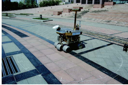
Figure 8: The mobile robot mounted with the visual sun compass prototype and an IMU.
