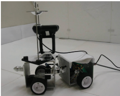
FIGURE 8: A general view of the built robot, including the docking connector and the visual system.
