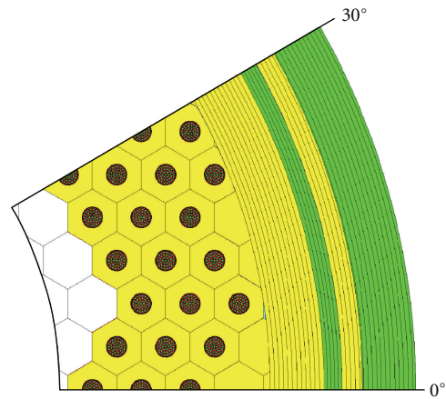
FIGURE 6: Scheme 1/24 of the reactor.
