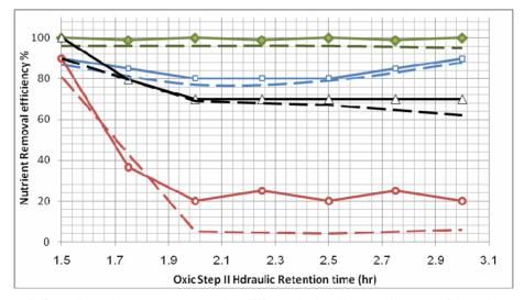
Figure 9. Overall nutrient percent removal at different hydraulic retention time of the oxic step II.
