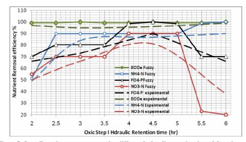
Figure 7. Overall nutrient percent removal at different hydraulic retention time of the oxic step I.
