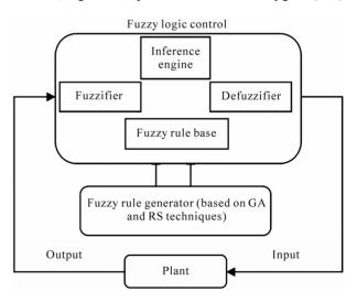
Figure 1. System configuration of RsFLC.
