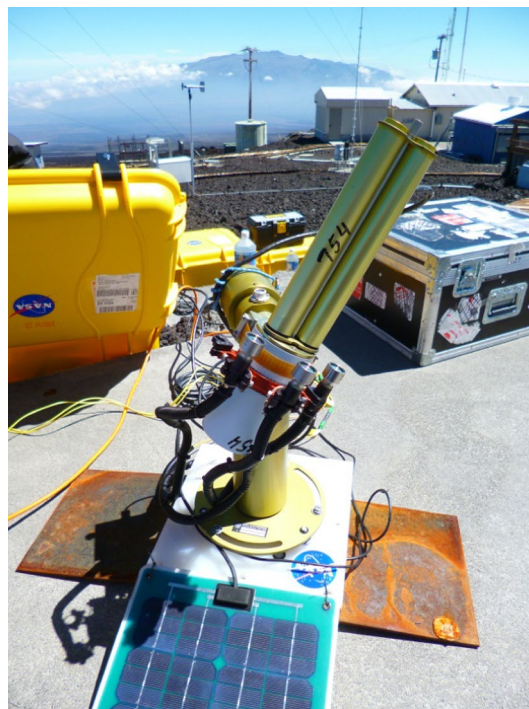
Fig. 3 Mini-LHR instrument is shown at the Mauna Loa Observatory in Hawaii. MLO is the site of the longest running measurements of atmospheric CO 2 , begun in the late 1950s by Charles Keeling. MLO offers a unique testing environment for the Mini-LHR, as the altitude helps ensure the atmosphere sampled represents the “background” signal of the atmosphere
