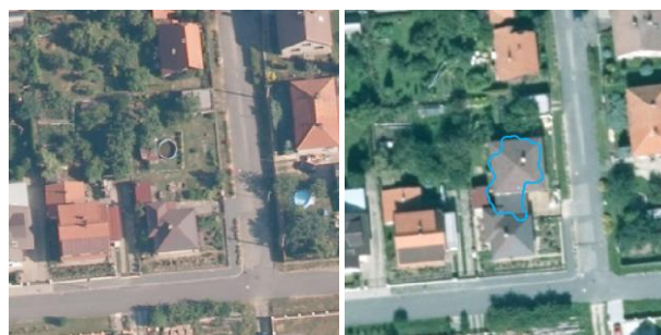
Figure 7. True indication of a new building
