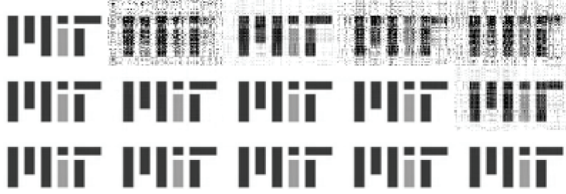
FIGURE 3: Recovered images under four measurement matrices with different numbers of linear constraints. From left to right: the original, results under Gauss, Binary, Sparse Binary, and Random Projection measurement. From top to bottom: p = 800 , p = 900 , and p = 1000 .
