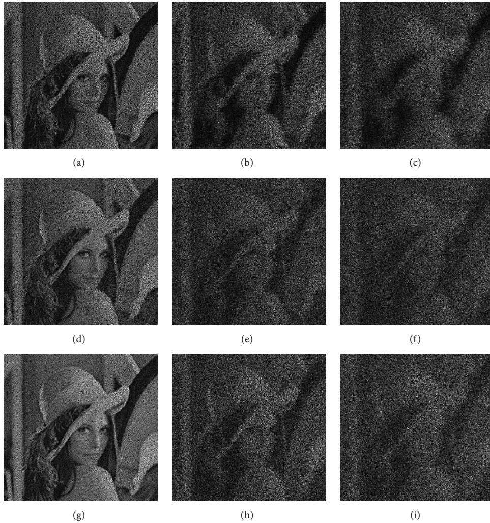
FIGURE 6: Results with incorrect parameters of FrT: (a–c) decrypted images with incorrect values of z_1 = 25.3, 26, and 27 mm, (d–f) decrypted images with incorrect values of z_2 = 35.3, 36, and 37 mm, and (g–i) decrypted images with variation in \lambda_p by 10, 20, and 40 nm.
