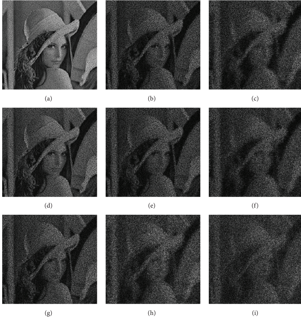
FIGURE 7: Results with incorrect parameters of DVTL: (a–c) decrypted images with incorrect focal lengths with deviation from correct value as 5, 10, and 50 mm, respectively, (d–f) decrypted images with incorrect \lambda with deviation from correct value as 10, 40, and 100 nm respectively, (g, h) decrypted images with incorrect topological charge with deviation from the correct value as 1 and 9, respectively, and (i) decrypted image with S = 2 .
