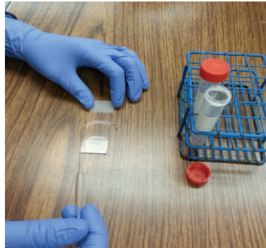
FIGURE 1: Spreading cells on a slide with a glass spreader. The glass spreader was made from a glass transfer pipette by heating it for a few seconds to minutes over an alcohol burner.
