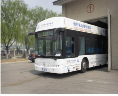
FIGURE 3: The range-extended electric bus developed by Tsinghua University.
