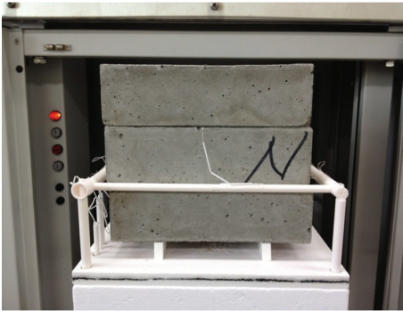
FIGURE 4: Thermal conductivity measurement of concrete bricks (230 mm × 114 mm × 65 mm) using hot wire (platinum resistance thermometer technique) [14].
