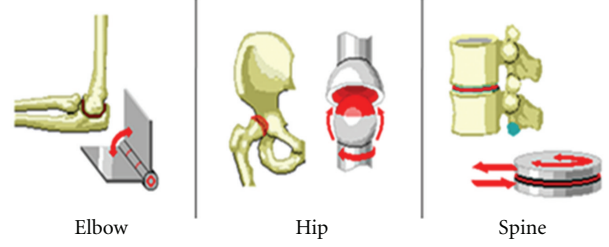
FIGURE 2: Human joints and their mechanical equivalent.
