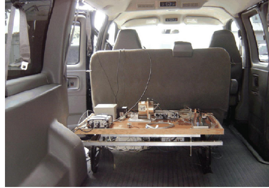
FIGURE 5: Equipment mounted inside the road test vehicle.
