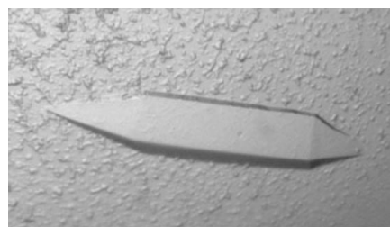
Figure 2 Crystal of BbCRASP-1 obtained by sitting-drop vapour diffusion. The crystal measures approximately 600 \mu m in length.
