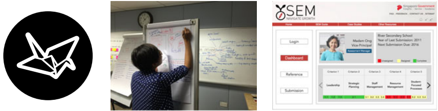
Figure 10. Example relaxed requirement prototype, (left) very low-fidelity and relaxed requirement prototype; (right) medium fidelity prototype. The design is for an evaluation tool that is used by multiple organizations. The prototype on the left allows for early, rapid prototyping of readability with the design team. While the higher fidelity, functional offline interface on the right allowed for testing with end users. Both are reduced fidelity prototypes, at different degrees.
