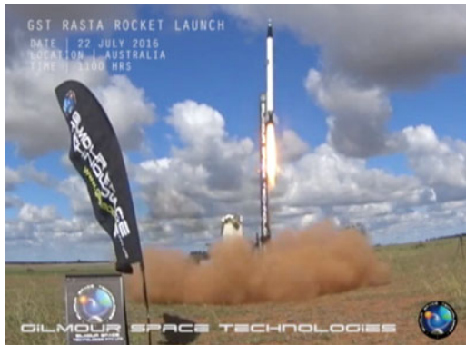
Figure 20. Launch of hybrid rocket using 3D printed, optimized fuel grains. Courtesy of Gilmour Space Technologies.
