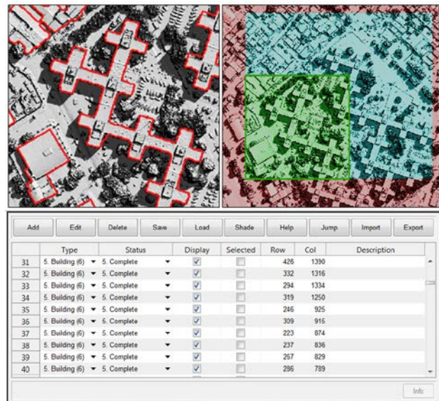
Figure 4 JHU/APL manual editing tool for building polygons includes a drawing window (top left), a context window (top right), and a polygon attribute table (bottom).
