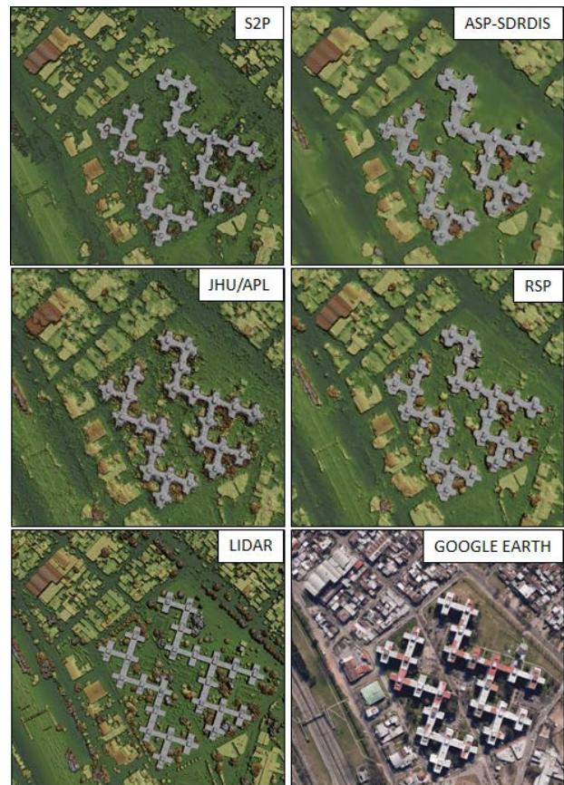
Figure 2 MVS and lidar point clouds are rendered as digital surface models and compared with Google Earth imagery.
