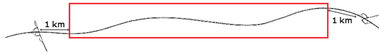
Figure 3 Simulated road section A5. Autobahn A5 south of Frankfurt, Germany. CAMs received within the boxed areas are used for the statistics.
